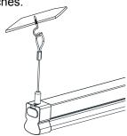
4. **Connecting the power cord** After installation, plug the power cord (B) into the end of light and then into the power supply.
