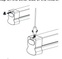
1 (B) **Mounting to wood** Drill a 1/16" diameter pilot hole in the ceiling. Make sure to fasten the combo wood-machine end into the metal hook. Tighten the hook screw into the wood.
